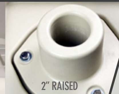
BUSHING Raised and flat reducer bushing. Raised design increases friction on post mount applications. 2"=2 1/2" ID. 4"=4 11/16" ID.
